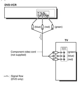
If your TV accepts progressive (480p) format signals, you must use this connection and then press the PROGRESSIVE button on the front panel when the DVD player is in stop mode to accept progressive video signals. The PROGRESSIVE indicator lights up in blue when the DVD player outputs progressive signals.
